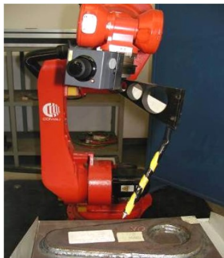
Fig. 5. Manual guidance device (Developed by CNR-ITIA for COMAU)
