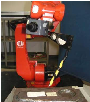
Fig. 2: Manual guidance device (Developed by CNR-ITIA for COMAU)
