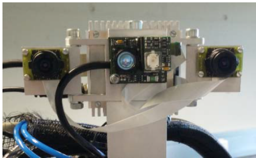
Fig. 4. Machine Vision systems mounted on the robot
