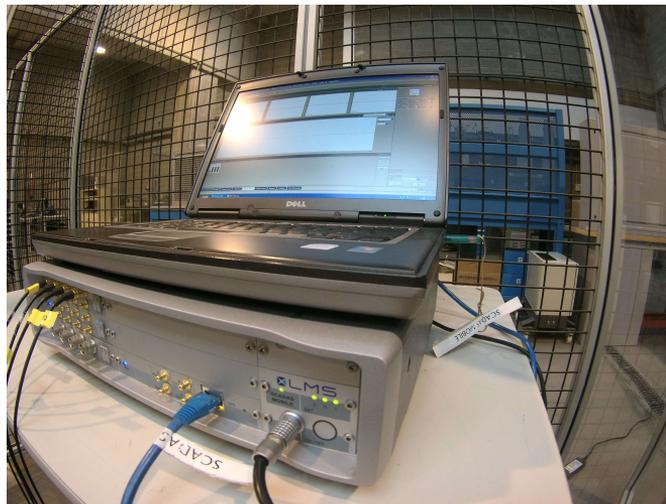
Figure 15.29: Siemenes LMS TestLab analyser
