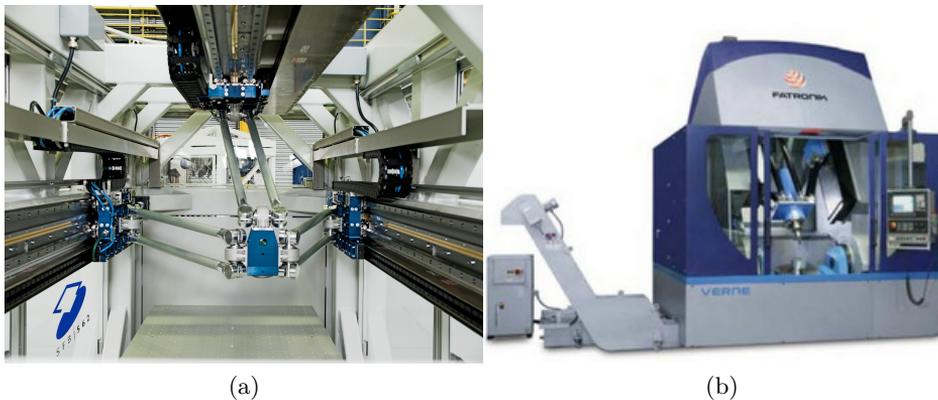
Figure 1.21: Two machine centres with PKMs: (a) Cosmo Center PM-600. Courtesy of Okuma; (b) Vertical Turning Machine V100. Courtesy of Index
