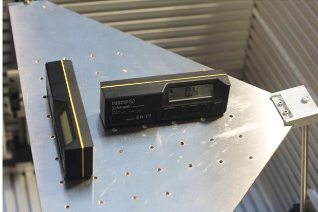
Figure 14.17: Inclinometers to measure the real position
