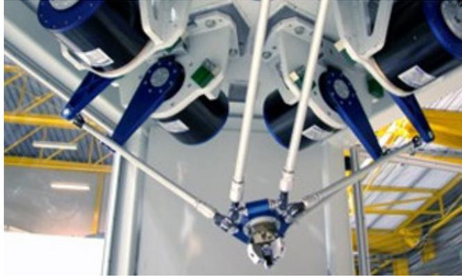
Figure 1.20: Hexa 6-DOF parallel manipulator
