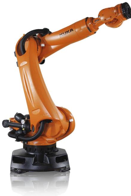
Figure 1.5: 6-axis serial robot. Courtesy of KUKA Robotics
