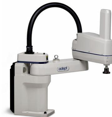
Figure 1.4: SCARA robot. Courtesy of Adept
