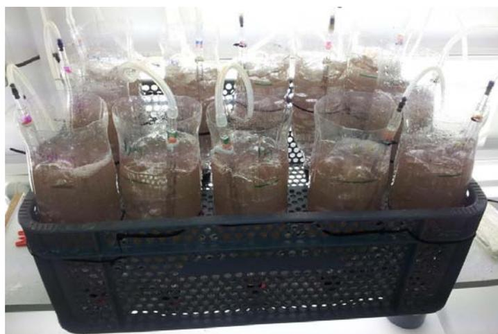
Figure 4- Reactors made from 1.5 L plastic bottles with the brine shrimp culture and continuous aeration.
