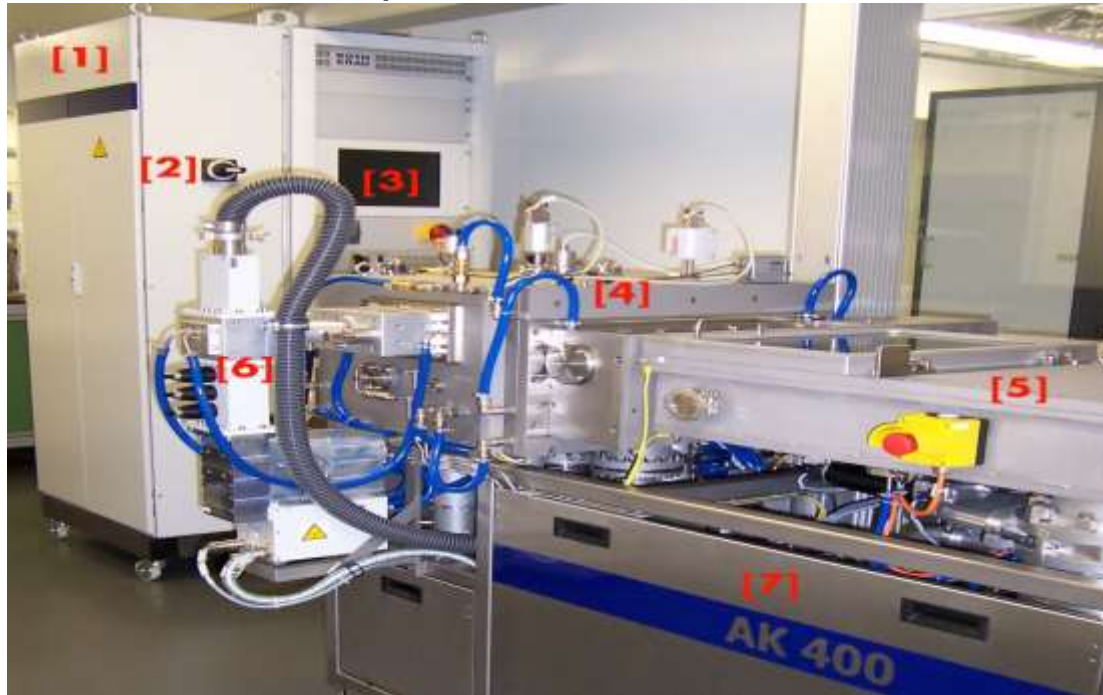
Figure 5.4 Description of PECVD machine used deposit SiNx layer
