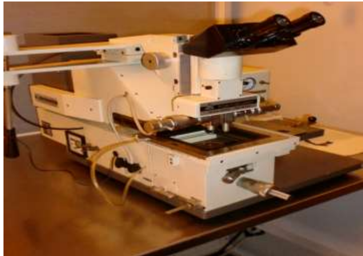
Figure 3.31 Photolithographic machine used in photolithographic step for front contacts.
