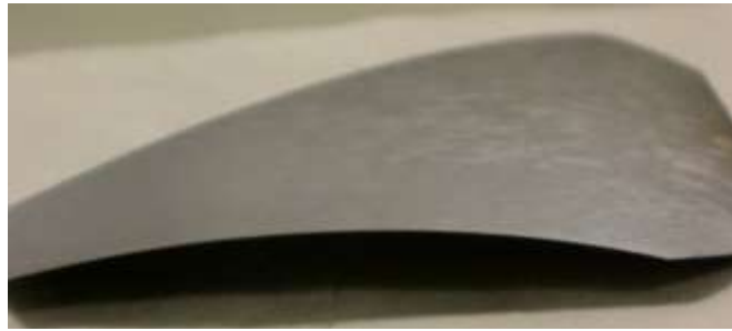
Figure 3.27 Wafers are bended due to Al diffusion at high temperature
