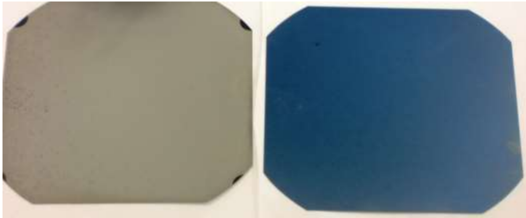
Figure 3.30 Front and back side of silicon wafers after drive-in and AR coating.
