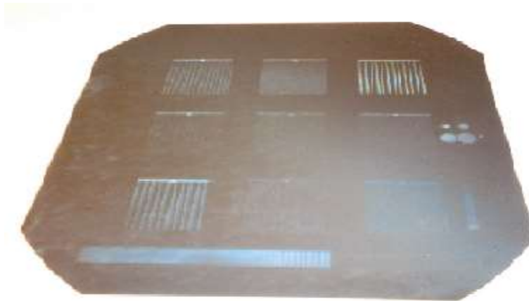
Figure 3.32 Image of wafer after development of photoresist
