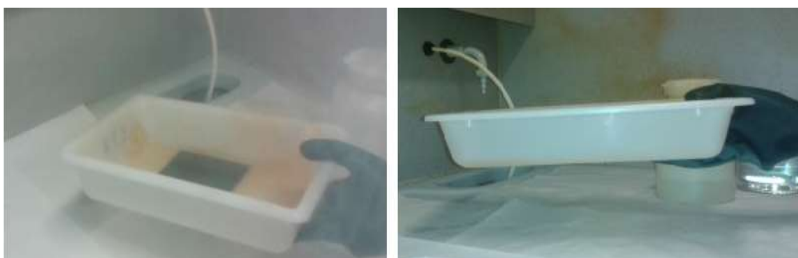
Figure 5.15 CPX manually etching process for silicon wafer.
