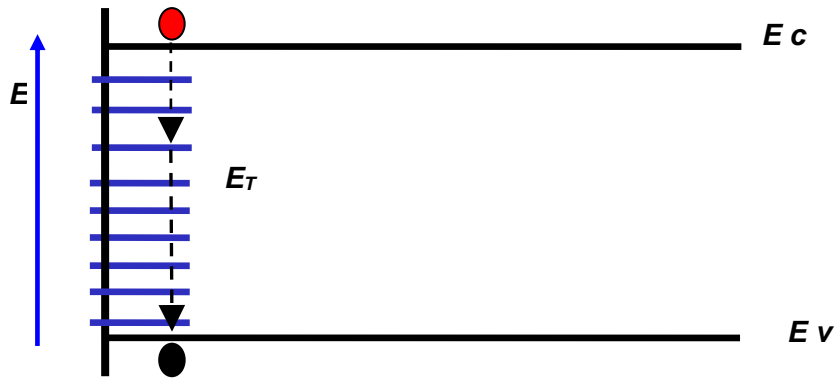
Figure 2.24 Energy band diagram representing SRH recombination through surface defects in the band gap
