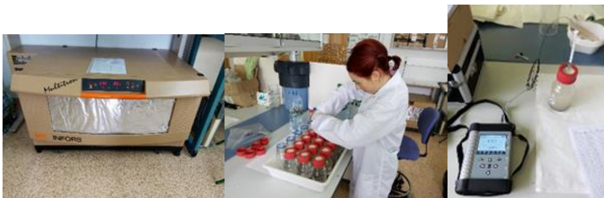
Figure 3: Set up and equipment used for the microbial respiration measurements using bottle incubations.
