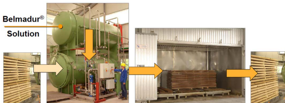
Figure I-28 Stages of Belmadur process (BASF pilot plant, Gottingen, Germany). Adapted from H. Millitz presentations.
