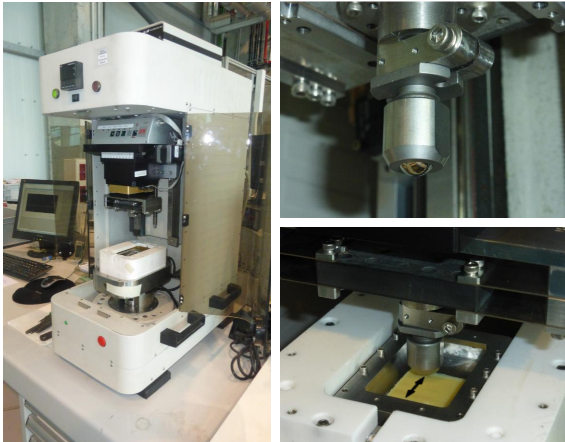
Figure 6.2. Linear Reciprocating Tribometer at IK4-Tekniker.
