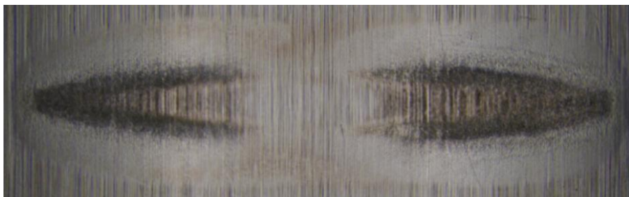
Figure 3.3. Microscopy of a false brinelling damaged bearing raceway (courtesy of Fabian Schwack).
