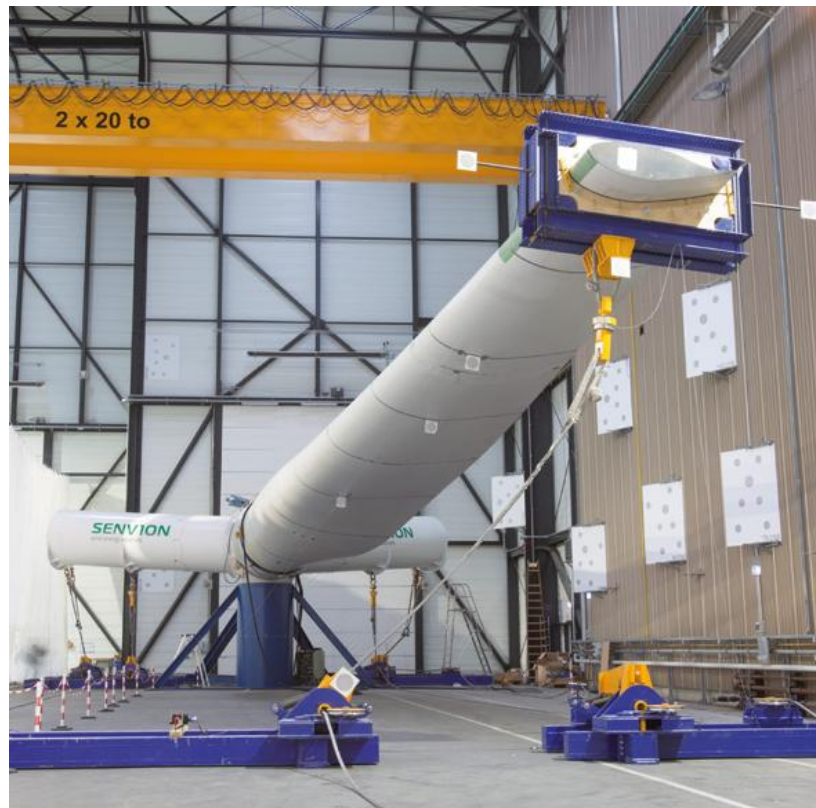
Figure 1.16. Pitch bearing test rig at Fraunhofer IWES [96].
