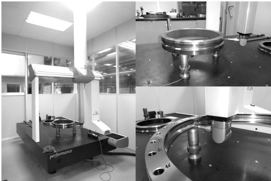
Figure 2.2. Coordinate-measuring machine and measured rings.
