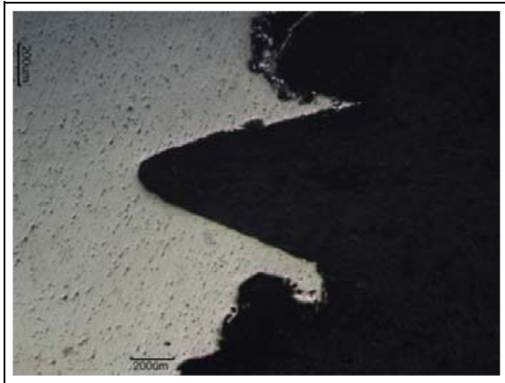
Figure 17. Pits on the probe with MG condition.
