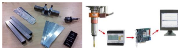
Figure 4. a. Sheets (Al), tubes (AISI1045), tools and fixture for the friction drilling process; b. Force-torque measurement with Artis©
