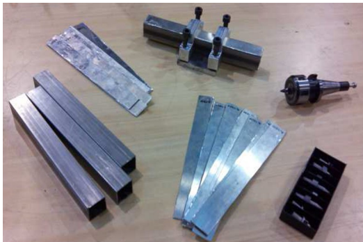
Figure 2. Workpiece: sheets, tubes and clamping adaptor for the forming processes
