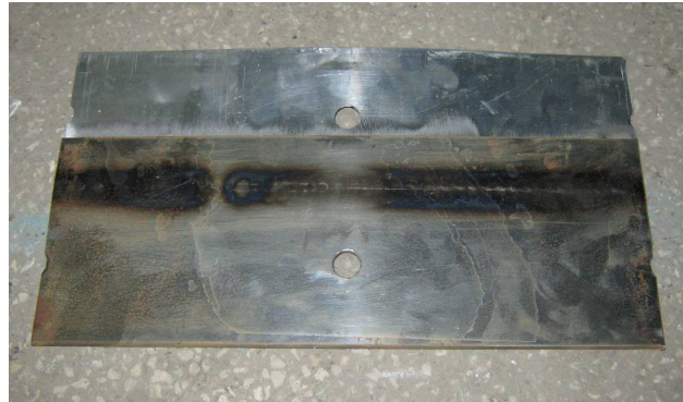
Figure 13.b. Rear view of the FSW joint test sample P11 [2]
