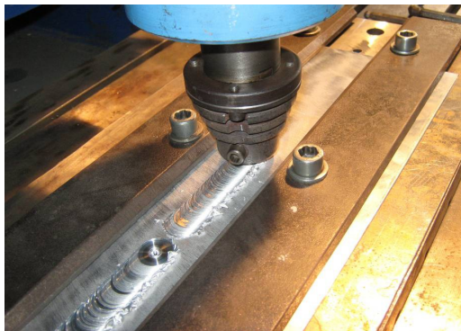
Figure 11. Running the FSW joining test P11, on the P11.2 segment [2]
