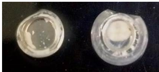
Figure 3-21. Opened Tzero pan with 10 mg of sample after measurement. The presence of sample on the lid is clearly observed.
