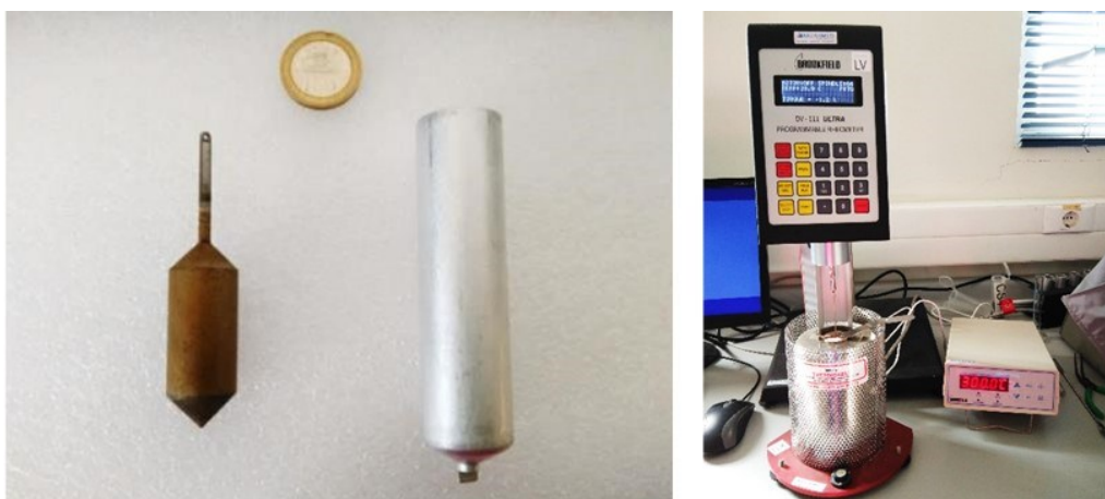
Figure 3-16. Left: The spindle and the sample chamber used for the rheological tests (Rheometer 1). Right: General view of the rheometer. The spindle is hung on the device which applies the rotational force and then immersed into the molten salt contained in the sample chamber.
