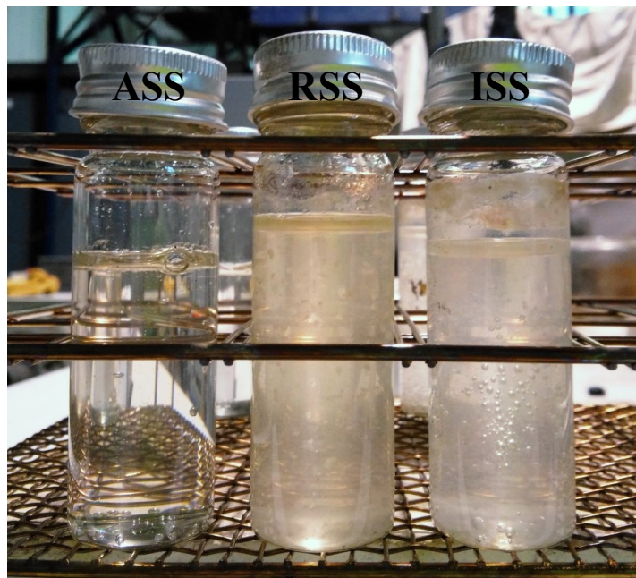
Figure 7-1. Visual appearance of the three Solar Salts in the molten state (396 °C). ASS (left), RSS (middle), ISS (right). Solid impurities are clearly seen in RSS and ISS.
