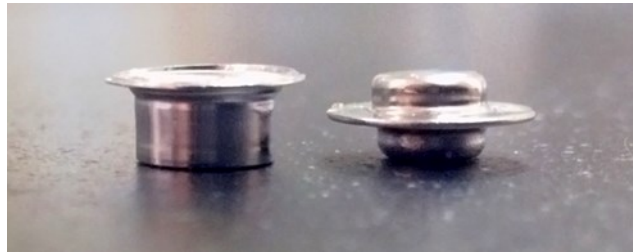
Figure 3-19. T-zero crucibles (left) and traditional crucibles (right). Both are hermetic and made of aluminium.
