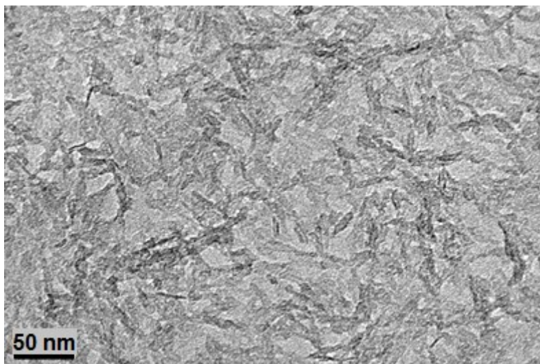
Figure 3-52. TEM image of the alumina nanoparticles.
