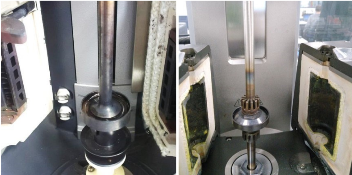
Figure 8-4. The rheometers with the parallel plate configuration. Rheometer 2: AR 2000ex (left) and Rheometer 3: MCR 302 (right).
