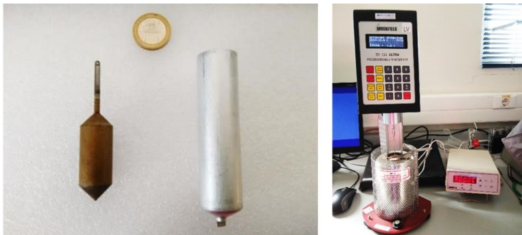
Figure 8-3. Left: The spindle and the sample chamber used for the rheological tests (Rheometer 1). Right: General view of the rheometer. The spindle is hanged on the device which applies the rotational force and then immersed into the molten salt contained in the sample chamber.
