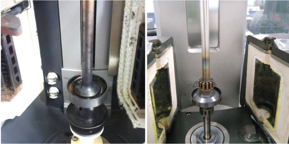
Figure 3-17. The rheometers with the parallel plate configuration. Rheometer 2: AR 2000ex (left) and Rheometer 3: MCR 302 (right).
