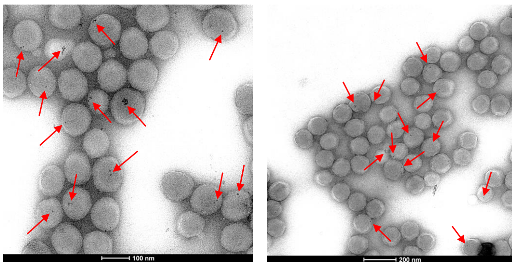
Figure 2.12 TEM micrograph of hybrid PS-QD/PMMA polymer particles of Run CS2.
