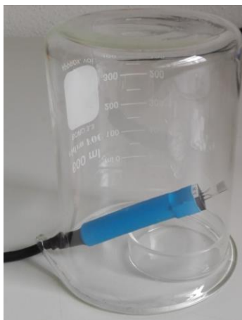
Figure 5.20 D03E24 electrode into an acetone steam-rich atmosphere prepared for the resistance measurements. (Property of Tecnia. All the rights reserved)
