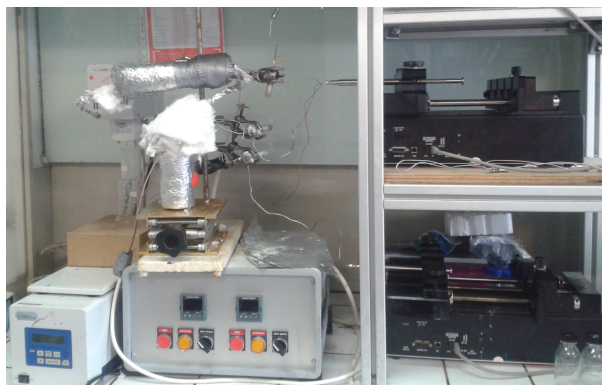
Figure 3.2 Picture of the experimental set up used for the synthesis of CdSe core and CdSe/CdS core-shell quantum dots.
