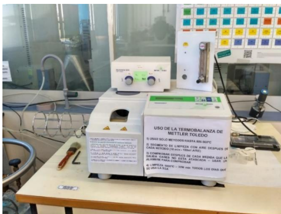
Figure 2.16. Photography of a TGA Mettler Toledo 822 e module
