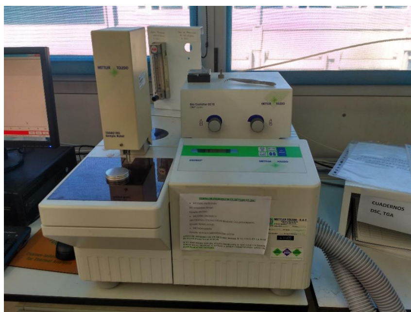
Figure 2.18. Photography of a DSC 822 e module
