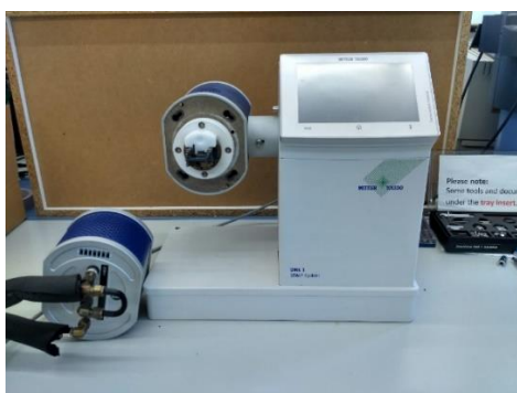
Figure 2.19. Photography of Mettler Toledo DMA1 (a) and TA-Instruments DMA Q800 (b)
