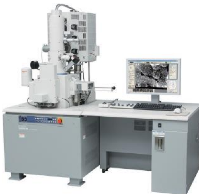
Figure 2.23. Photography of Hitachi S-4800 field emission scanning electron microscope (FE-SEM)
