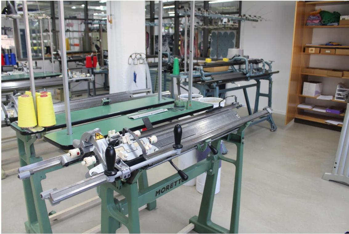
Figure 6.4. Knitting machine used to produce fabrics
