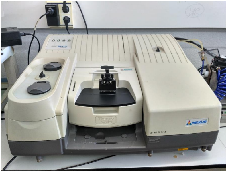
Figure 2.14. Photography of a Nicolet Nexus FTIR spectrophotometer
