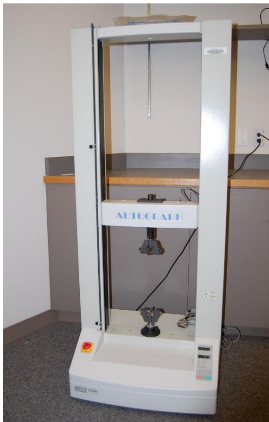
Figure 2.26. Photography of Shimadzu Autograph (a) and Tinius Olsen H10KT (b)
