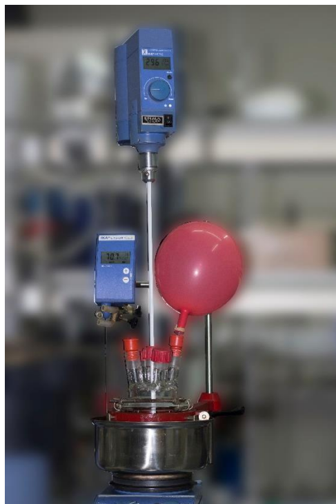
Figure 2.8. Equipment for synthesis of shape memory polyurethanes
