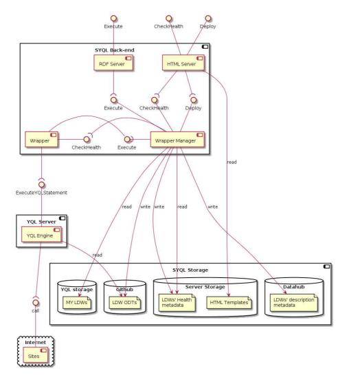
Figure A.6: SYQL back-end components diagram (simplified SYQL storage component)
