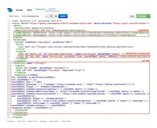
Figure 4.5: YQL Editor Console. Turning the ODT in Figure 4.3 into an LDW
