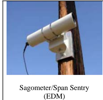
Figure 8. Commercial system based on sag monitoring
