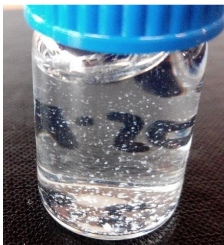
Figure 4. Aspect of the dispersion recovered after the emulsion polymerization of VCL using KPS as initiator, \text{NaHCO}_3 as buffer and \text{P}(\text{AETAC-X})_{76} as stabilizer (expt 6, Table 3 ).
