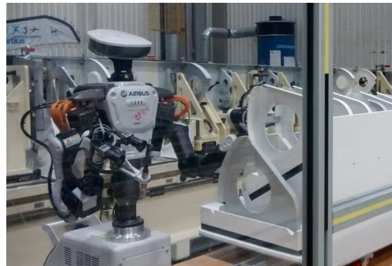
Fig. 6: Pilot station at Airbus facilities deburring rib drillings
