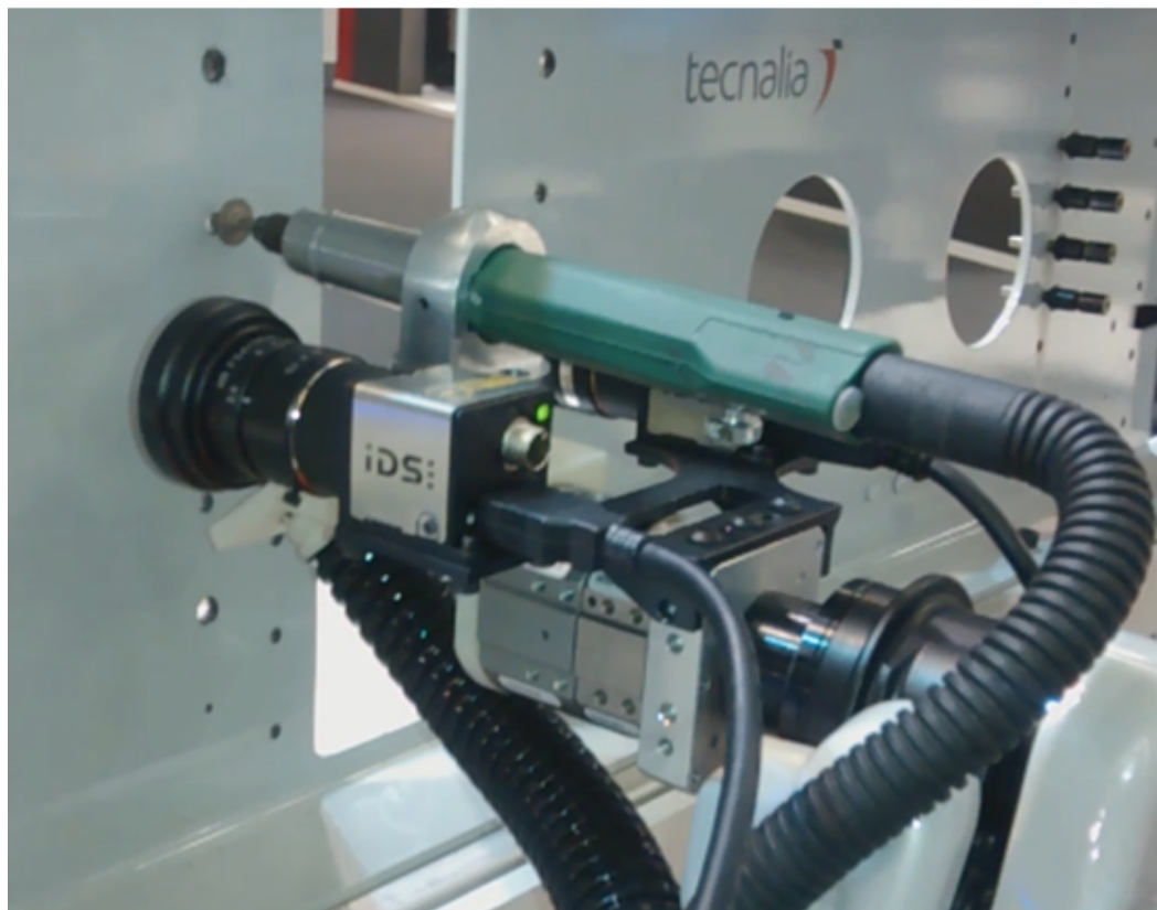
Figure 7.6: Deburring a drilling based on the vision result
