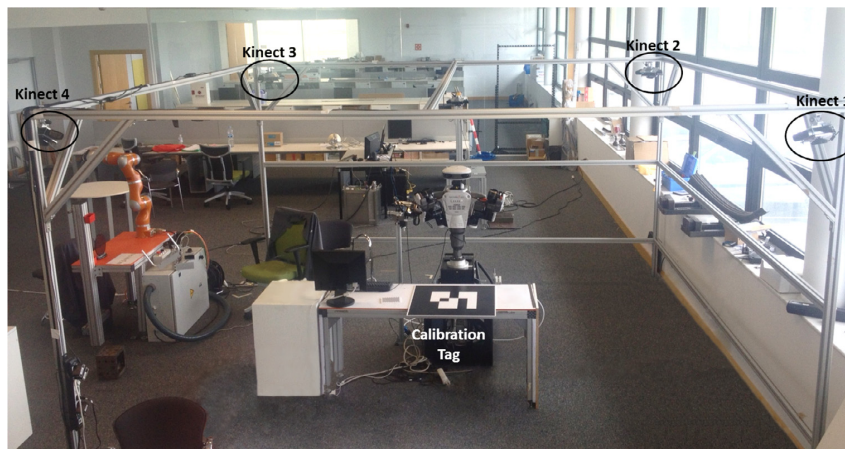
Fig. 7. Location of the RGBD sensors for Workspace Monitoring.
