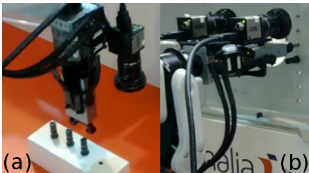
Figure 7.7: Picking and inserting the rivet into a drilling
