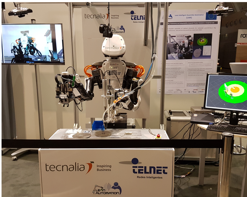
Figure 7.17: Nextage robot performing antenna assembly operations
