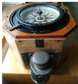
Figura 3.1 Compás acimutal Dumoulin Froment.
