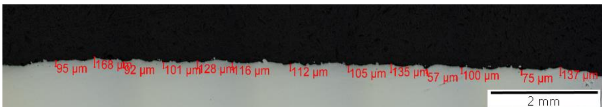
Figure 17 E.III-10 metallography: 1800 W and 0.25 mm/u feed forward.
