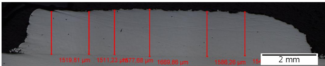
Figure 14 E.II-17 metallography: 2400 W laser power and 0.25 mm/u feed forward and 0.23 mm ND.
