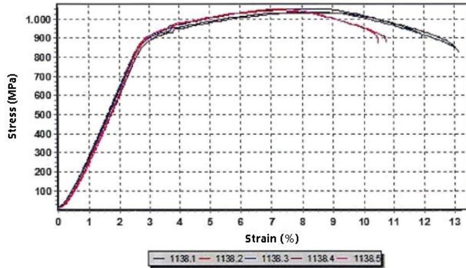
Figure 56 4340 10 mm build up with cooling stress-strain curve.
