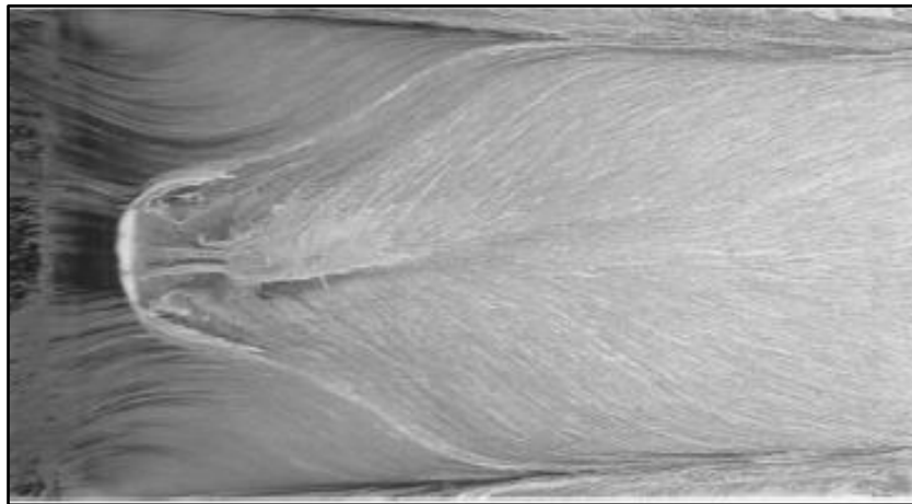
Figure 9: Flow visualisation of diffuser ramp at 20 degrees. Flow from left to right. Reproduced from [16]
