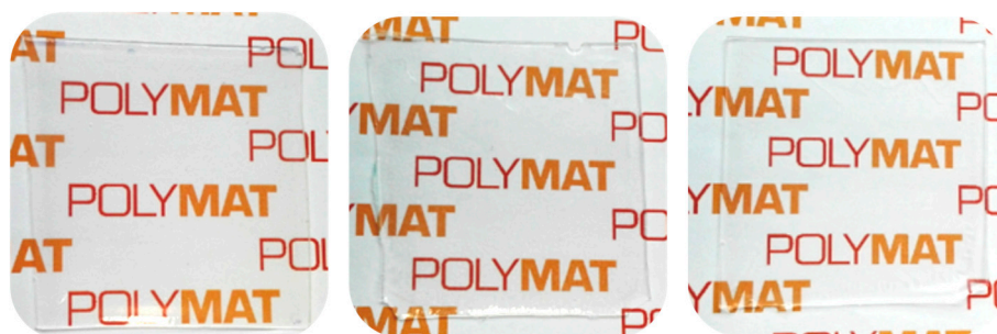
Figure 7. Pictures of polymer films containing (from left to right) 20, 30, or 40 wbm% methacrylate fructose.
