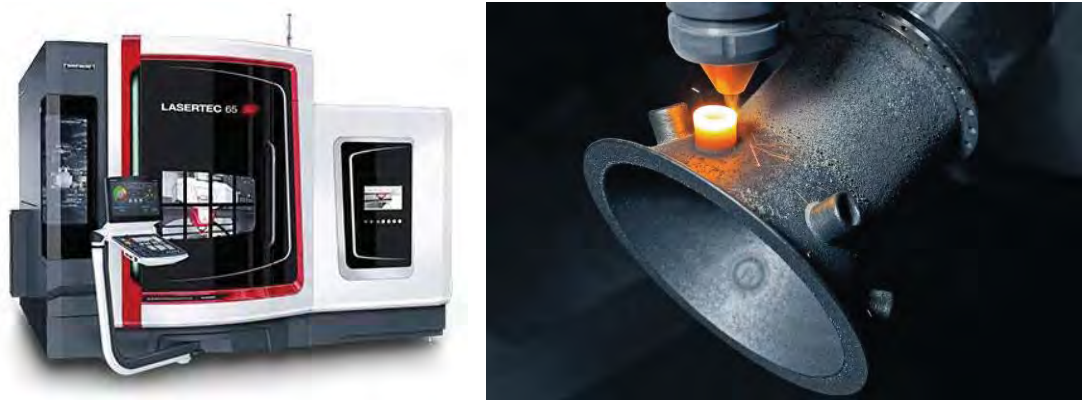
Figure II. 19: The hybrid machine LASERTEC 65 3D developed by DMG-Mori (left) and an additive operation (right) [DMG Mori, 2017].
