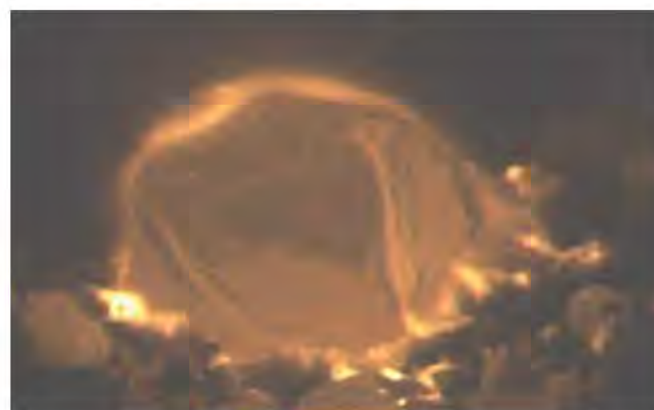
Figure II. 84: Screenshot of the melt pool for a Gaussian intensity distribution laser beam [Gibson, 2009]
