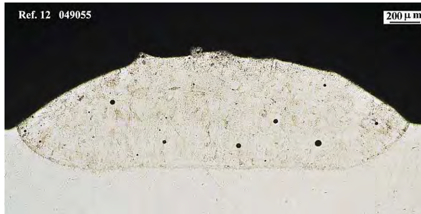
Figure II. 44: Appearance of pores in an AISI 316L clad.
