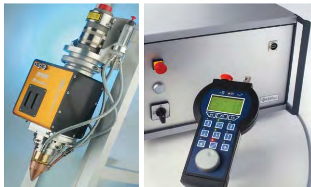
Figure II. 40: LMD processing head VarioClad (left) and the control unit (right) [Reis, 2017].
