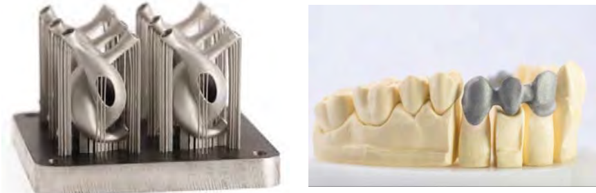
Figure II. 10: An Aorta pendant on small build plate with supports (left) and an image of a SLM manufactured bridge model (right) [Renishaw, 2017].
