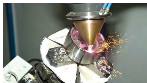
Figure II. 41: The continuous coaxial nozzle YC52 from Precitec [Precitec, 2017].
