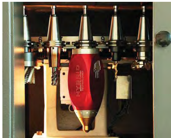
Figure II. 42: The LMD nozzle Ambit™ from Hybrid Manufacturing Technologies [Ambit, 2017].
