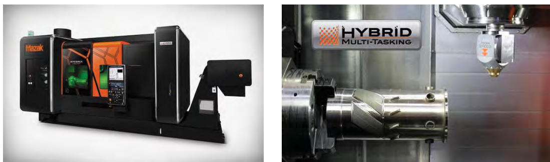
Figure II. 20: The hybrid machine Integrex i-400AM developed by Mazak (left) and a demonstration part (right) [Mazak, 2017].
