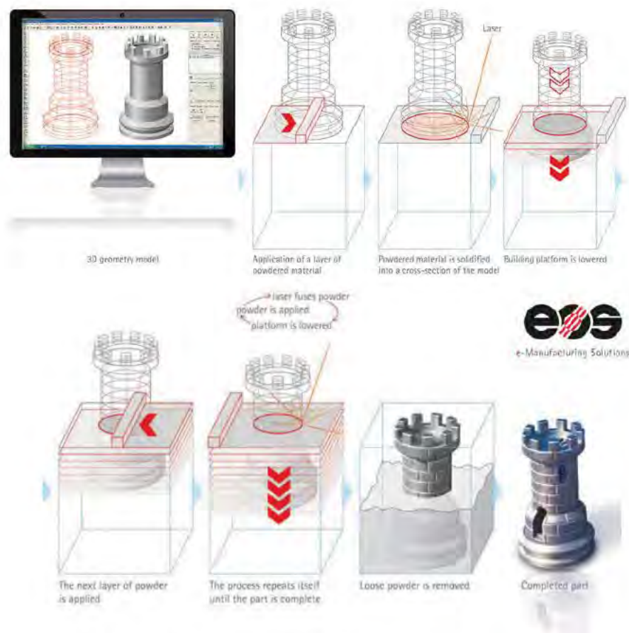
Figure II. 8: General function principle of laser sintering [EOS, 2017].
