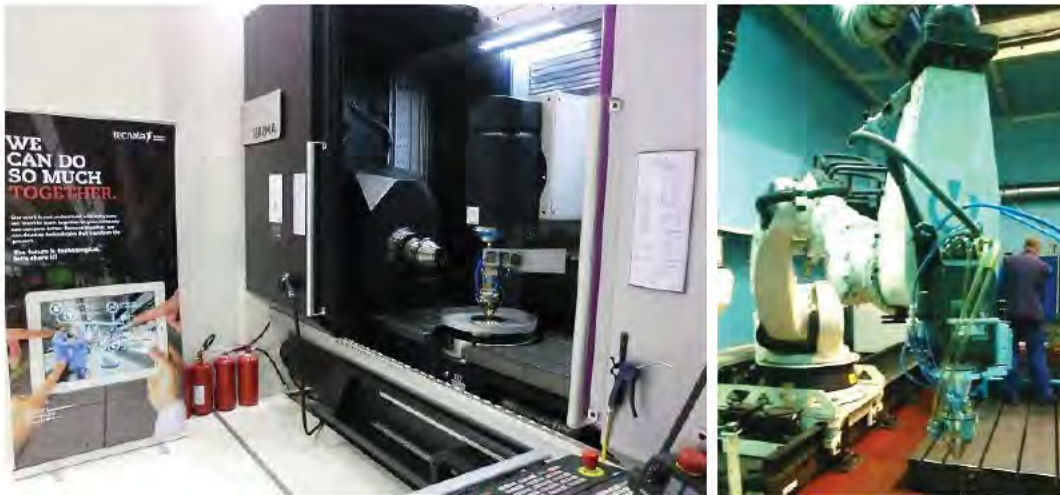
Figure II. 12: Different alternatives for LMD systems, a Cartesian hybrid machine from Ibarmia (left) [Ibarmia, 2017] and an anthropomorphic robot (right).
