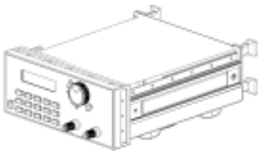
Fig.1-2 Front view of 3700 Series DC electronic load
