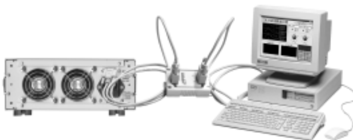
Fig.1-1 Connect the electronic load to PC
