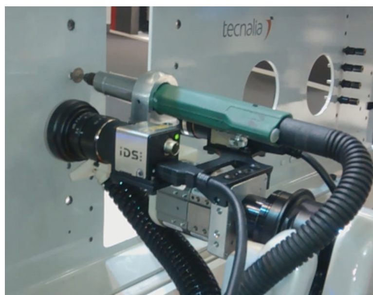
Figure 8. A drilled hole is deburred after detecting its position by vision.
