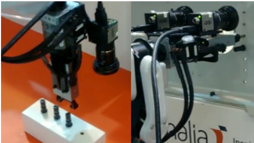
Figure 9. (a) The right arm of the robot is taking a rivet from a tray; (b) after taking the rivet, it is introduced in the previously-detected drilled hole.
