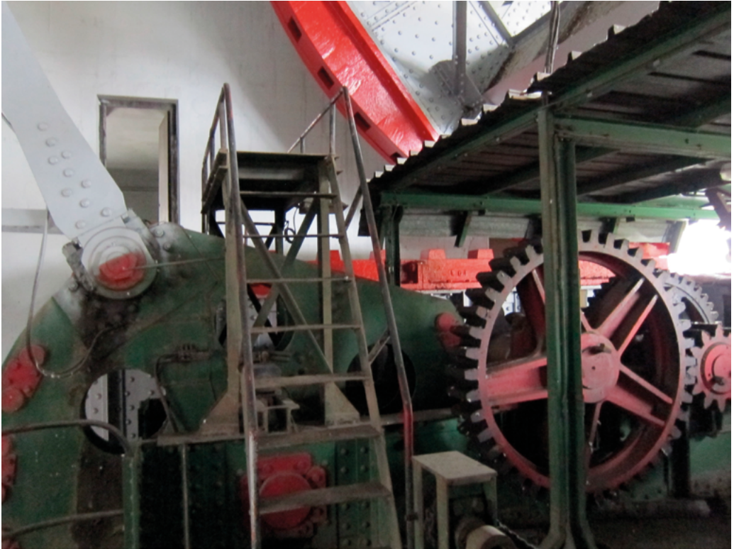
Figure 4.14. Part of the machinery of the Deusto drawbridge.
