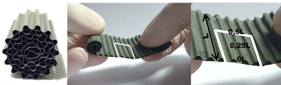
Figure 3. Illustration of the studied area of each monolith for SEM and EDX.
