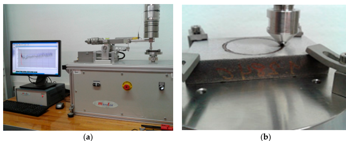
Figure 2. Pin-on-disk laboratory test equipment used for the experiments (a) and detail of the wear track created by the turning the tungsten carbide (WC) counter ball over the sample surface (b).
