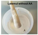
**Figure 5.4.** Visual appearance of the final waterborne paints prepared using the latex synthesized without any functional monomer.
