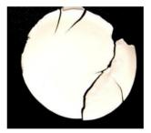
Figure 3.19. Paint-like film produce using PCC at the PVC value of 45, with the latex of 120 nm.
