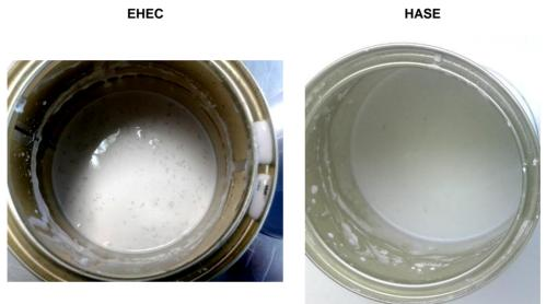
Figure 4.11. Paints prepared with MAA/BA/AA latex at the PVC value of 60, with the blend of the three calcium carbonates and with TiO<sub>2</sub>. In the left using EHEC thickener and in the right HASE thickener.
