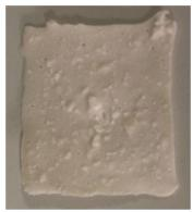
Figure 3.2. Waterborne paint-like film prepared without additives, PVC 45, SC 65%.
