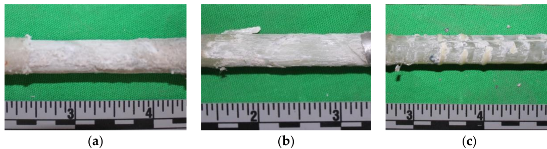
Figure 7. Bond surface of the GFRP rebar after completion of the bond test: type A (a), type B (b) and type (c).
