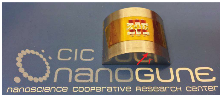
Figure 5.1| A sample holder. The photography shows a bent flexible chip on Kapton with six i-MOS devices. The sample is pasted on a half cylinder that works as sample holder and that permits performing measurements under applied strain.
