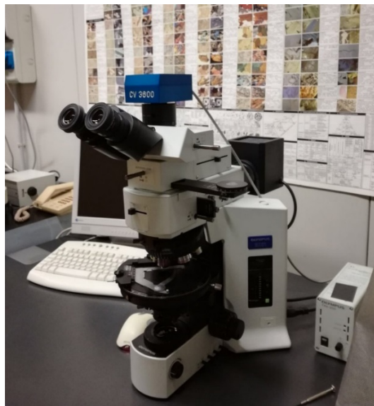
Figure 3.9. Olympus BX 51 petrographic microscope.
