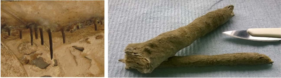
Figure 3.5. Calcium carbonate stalactite-like formations (FLG) collected from the ceiling of the Lower Gallery (left). Details of the stalactite-like formations (FLG) (right).
