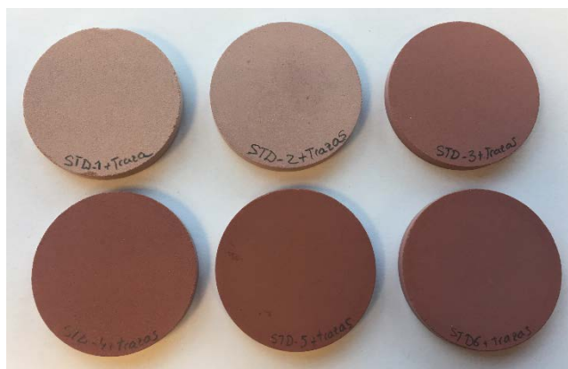
Figure 6.1. XRF synthetic calibration standards pellets.
