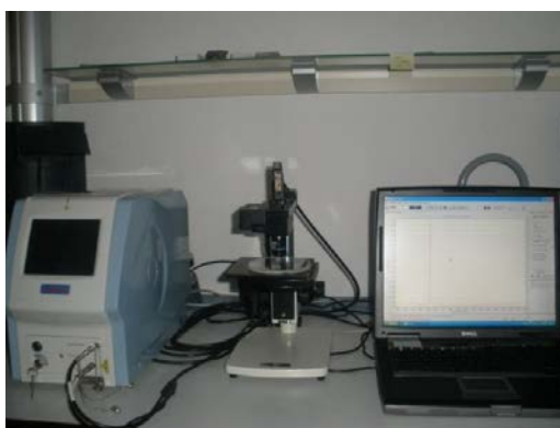
Figure 3.12. The portable innoRam™ Raman spectrometer with the probe coupled to the video-microscope.
