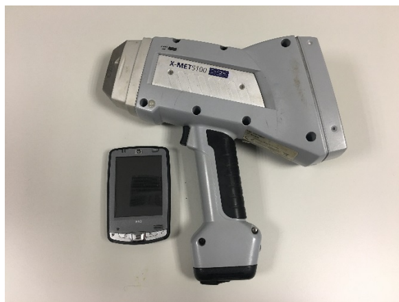
Figure 3.14. The XMET5100 HH-ED-XRF and its PDA disconnected from the device, which can be coupled to the spectrometer in the back part.
