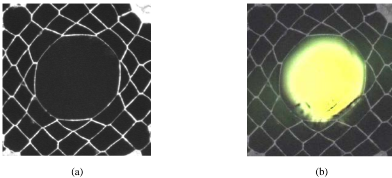
Figure 3.2 Photograph of the Kagome HC-mPOF. (a) Structure. (b) Structure when light is confined.
