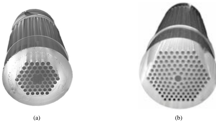
Figure 3.6 Photograph of the preforms. (a) 3R HC-mPOF. (b) 6R HC-mPOF.
