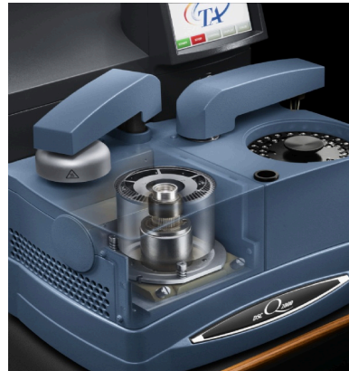
Figure 2.9: Left, a standard DSC thermogram where the change of the heat flow corresponding to the MT and magnetic transition can be observed. The inset shows the T_c transition in more detail. Right, the picture of the TA Q2000 DSC setup.
