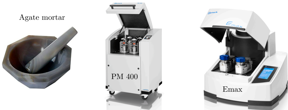
Figure 2.2: From left to right, an agate mortar, a planetary ball mill PM400 and Emax mill. Credit: Retsch
