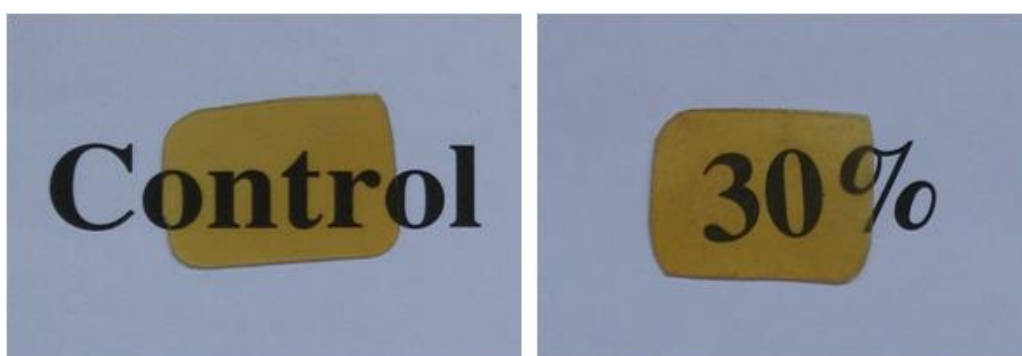
Figure 8.5. Photographs of the control film (CH0) and the film prepared with 30% chitin (CH30).
