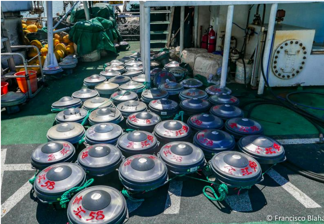
Figure I.15. Echo-sounder buoys on the deck of a purse seine vessel. Source: Francisco Blaha
