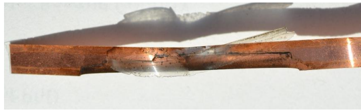
Figure 51: Foil electrode with an insulation layer of 22 \mu\text{m} .
