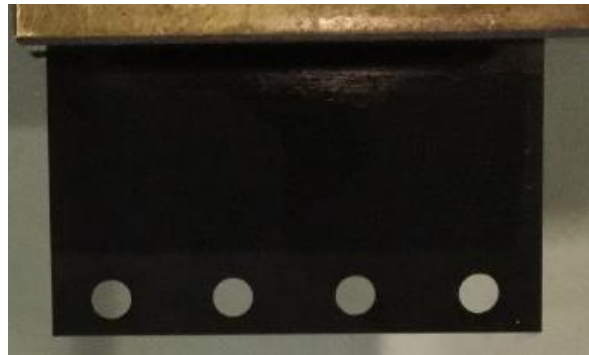
Figure 65. Specially designed graphite electrode for slot machining.
