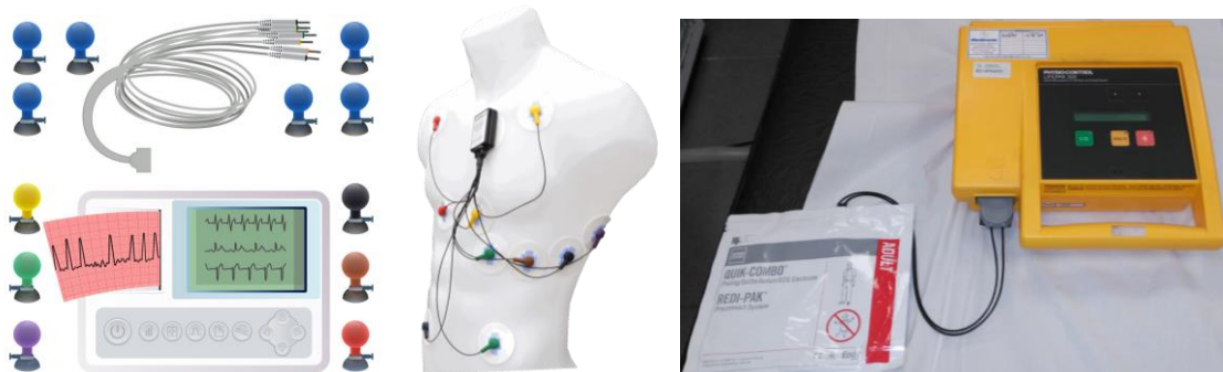
Figure 5: a 12-lead electrocardiograph (left) [20], a Holter (centre) [21], and a defibrillator (right).
