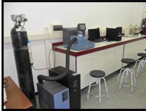
Figura 14: DSC TA Instruments Q200.
