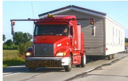
Figure 2.2.4 Transport of a modular single family home.
