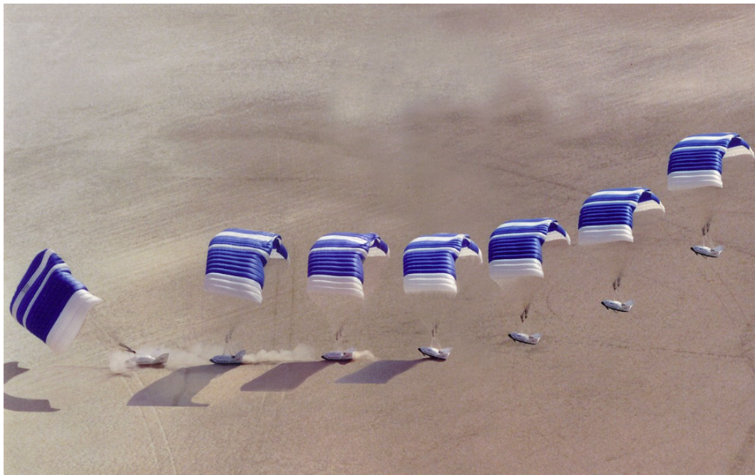
(c) A prototype X-38 emergency reentry vehicle approaching and landing with a large scale parawing (1999). Source: NASA
