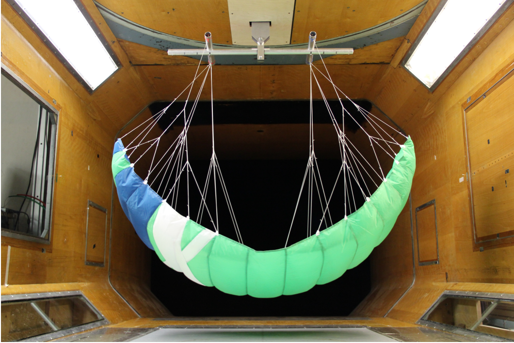
Figure 3.4: The kite hanged from the H frame inside the wind tunnel.
