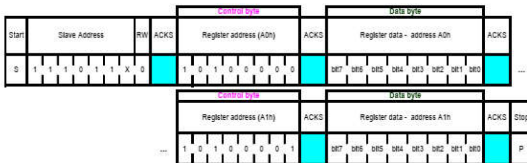
Figure 7: I 2 C multiple byte write (not auto-incremented)
