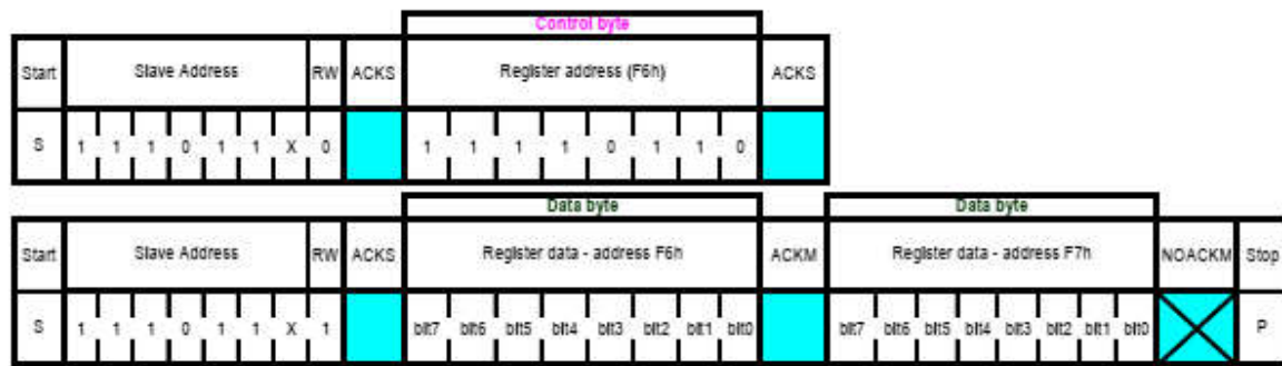
Figure 8: I2C multiple byte read
