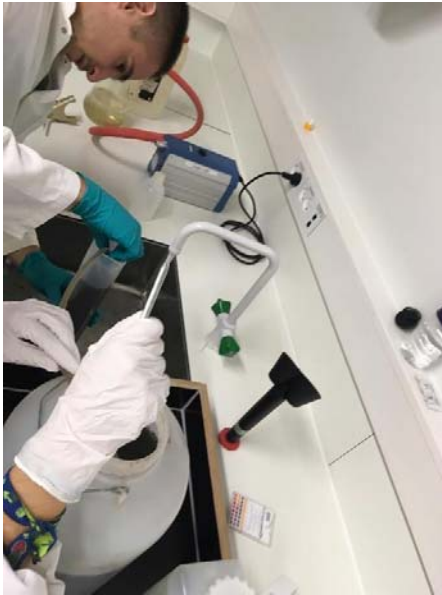
Figure II. 4. The activated sludge sample is put into the one-liter measuring glass by using a tube
