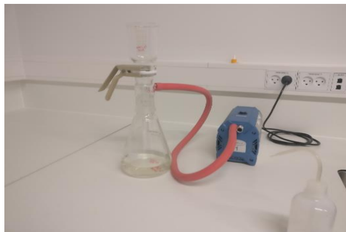
Figure II. 23. Filter de 50 ml sludge sample, by using the pred-dried filter
