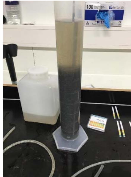
Figure II. 5. The activated sludge is settling till have of the volume is activated sludge
