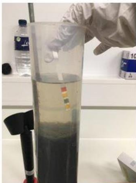
Figure II. 8. The pH of the sample is measured. Temperature is also measured.
