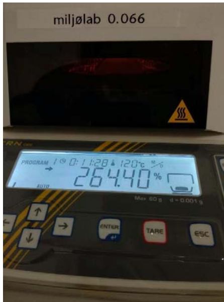
Figure II. 24. Dry the filter after the filtration and weigh the suspended solids on the filter paper
