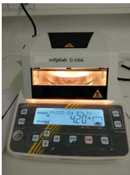
Figure II. 22. Dry and weigh the filter paper by using the weigh and dryer unit
