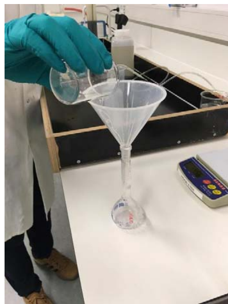
Figure II. 15. The 10 ml of the sodium nitrate solution is added to the one-liter sample
