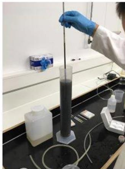
Figure II. 9. The sample has to be under slightly stirred conditions to keep it anoxic
