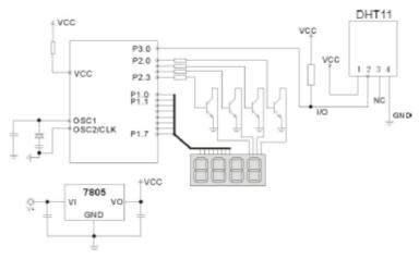
Microprocessor and DHT11 of connection typical application circuit as shown above, DATA pull the microprocessor I / O ports are connected.
