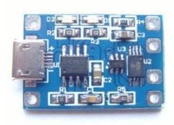
LC TP4056 Lithium battery charge and discharge protection module equipped with TP4056 chip, a maximum charge current up to 1.2A, and this module is equipped with a charge-discharge protection device for the voltage of 3.6V,3.7V, such as 18650, polymer etc., single or multiple parallel can also be used.
