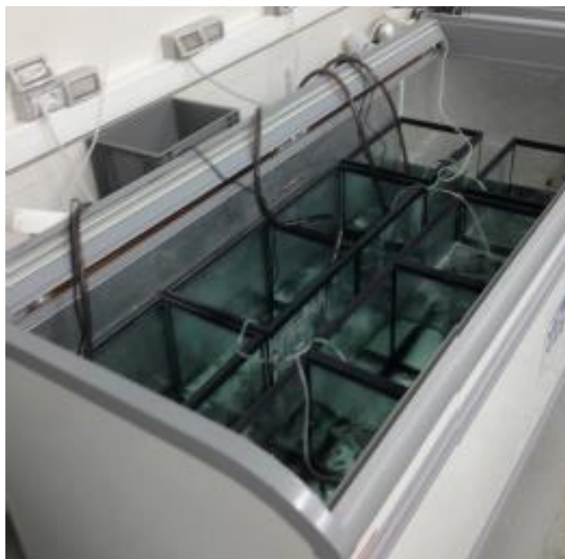
Fig. 3 The tanks set up in the refrigerators with the maintenance system
