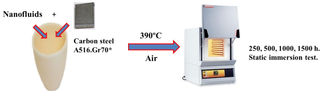
Figure 2.7. A scheme of the corrosion test protocol.
