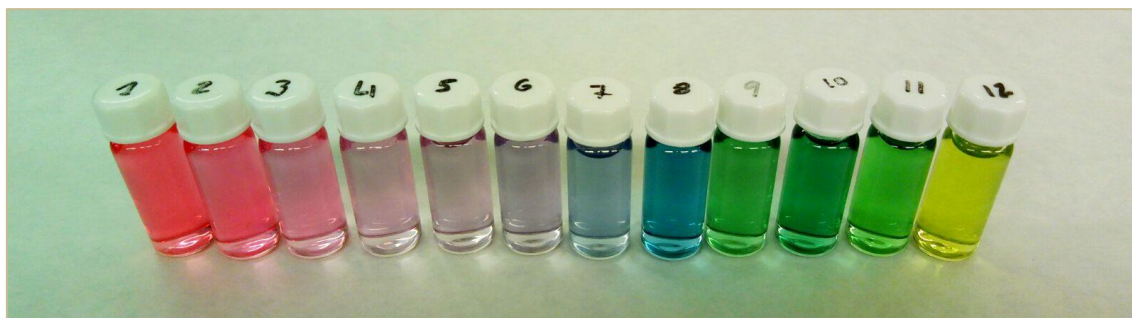
Figure 6.2 Colour change of anthocyanin solutions at different pHs (marked on the lids).
