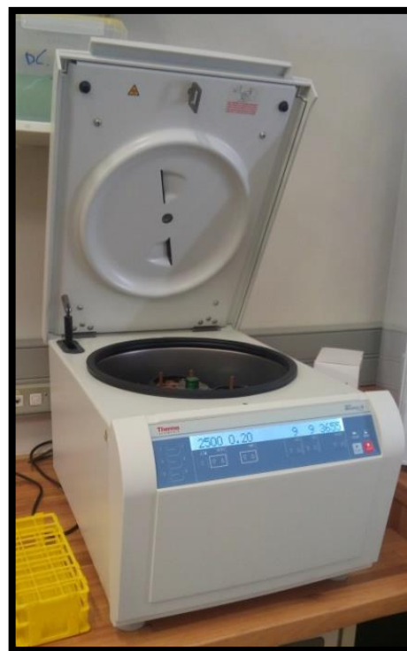
Figure 4.7: Thermo Scientific Heraeus Megafuge 16 used during the ultrafiltration process of the samples.
