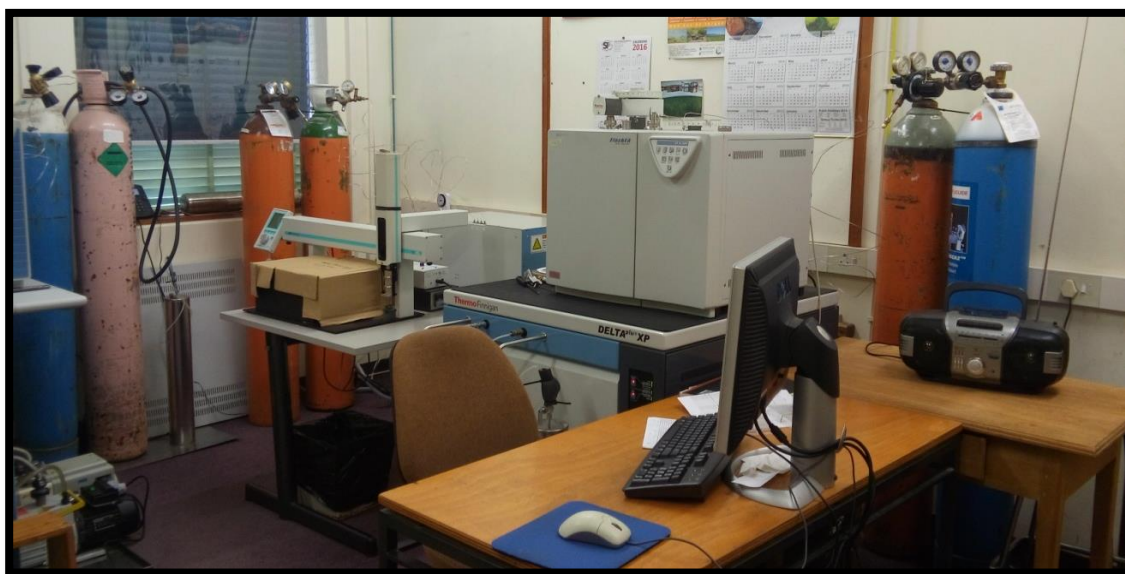
Figure 4.13: Delta plus XP continuous-flow isotope ratio mass spectrometer (Thermo Fisher Scientific, USA), interfaced with a Flash EA 1112 elemental analyser (Thermo-Finnigan, USA).
