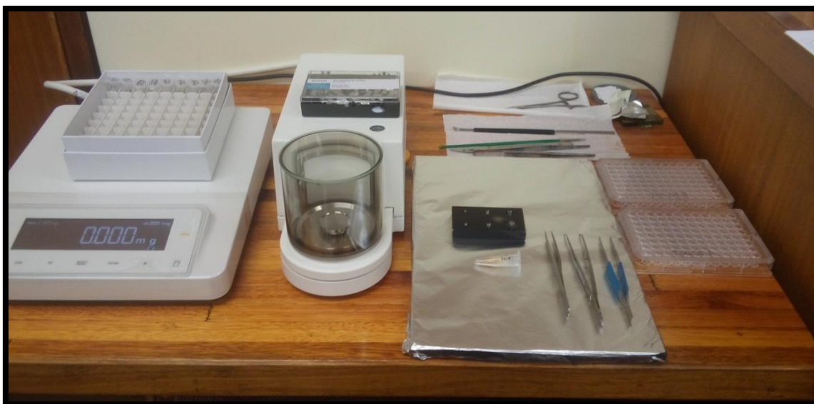
Figure 4.12: Microbalance used in the weight process of collagen into tin capsules.
