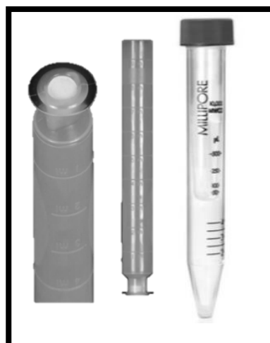
Figure 4.8: Eeze-filters and Amicon Ultra ultrafilter (30kDa).
