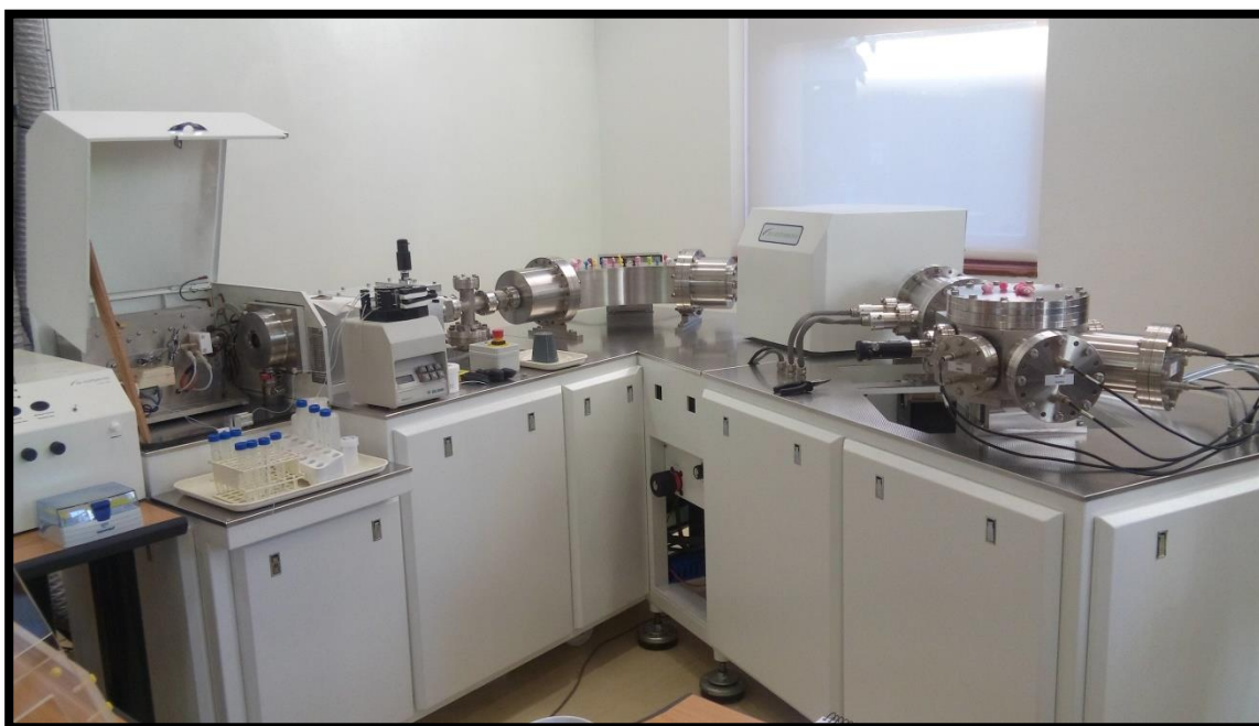
Figure 4.22: NuPlasma HR MC-ICP-MS. Department of Geology, University of Cape Town.
