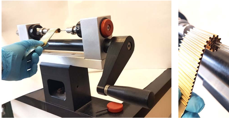
Figure 2.7. Equipment for rolling (left) and detailed image of two foils (corrugated and flat) assembled and rolled up (right).
