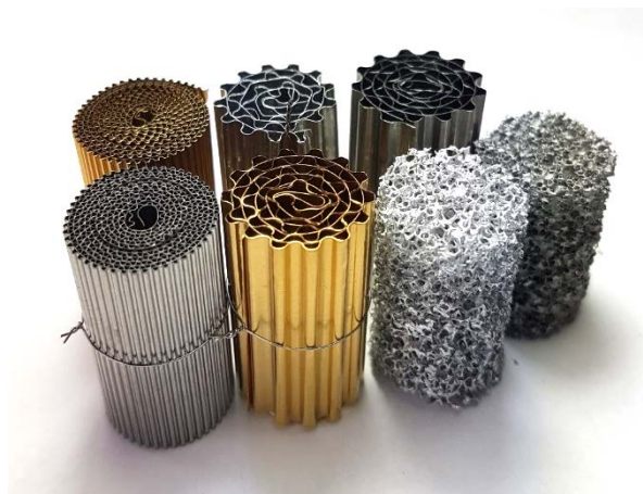
Figure 2.5. Metallic structured substrates used for structured catalysts preparation.
