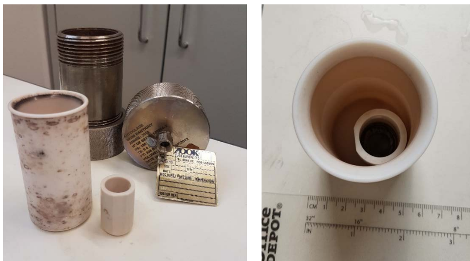
Figure 2.4. Autoclave and Teflon vessels used for zeolite synthesis with Cu@SiO 2 nanoreactors.
