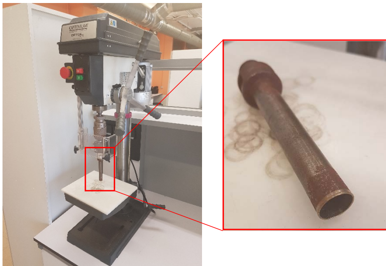
Figure 2.8. Photograph of OPTIdrill B 23Pro which is used to cut the cylindrical foam samples.
