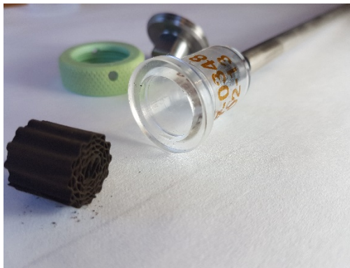
Figure 2.12. Autopore IV penetrometer for solid samples (5 cm 3 - Part No. 950-61707-00) and monolith with the required dimensions.
