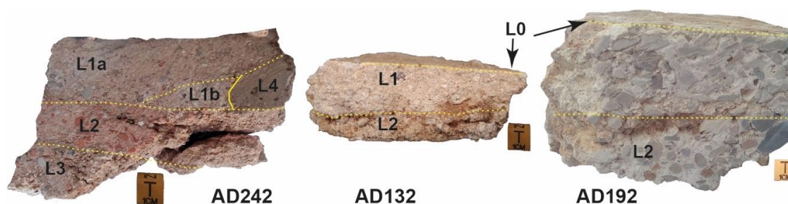
Figure 2. Representative samples of mortars from the Arroyo de la Dehesa de Velasco site. Sample AD-242: Multilayer wall plaster with cocciopesto layer. Sample AD-132: Two layers of wall siliceous plaster with an outermost marmorino layer. Sample AD-192: Multilayer floor mortar with three layers, L0 marmorino layer, L1 crushed limestone and L3 siliceous pebbles with calcite binder.
