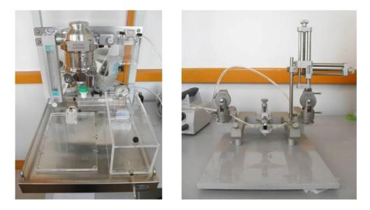
**Figure 3.16**: Left image: inhalation anesthesia system. Right side: mouse mask for anesthesia maintenance coupled to the inhalation anesthesia system shown on the left.
