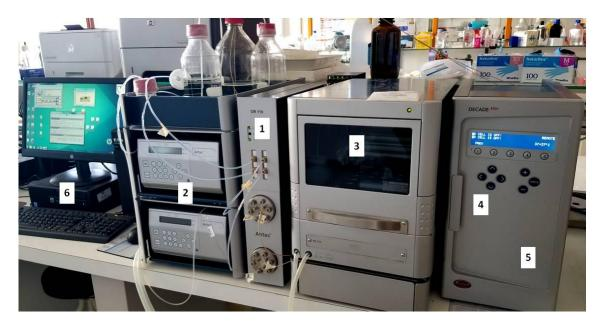
**Figure 3.25**: UHPLC equipment coupled to two electrochemical detectors. 1) Degasser; 2) Pump; 3) Autosampler; 4) Chromatographic columns; 5) Electrochemical detector; 6) Control station.
