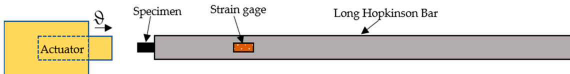
Figure 7. Schematic representation of intermediate strain rate compression test apparatus (Long Hopkinson bar setup).
