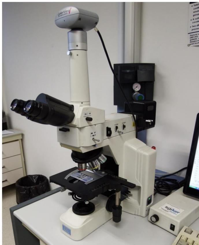
**Figure II-7 :** Microscope Electronique (Nikon Eclipse E600)
